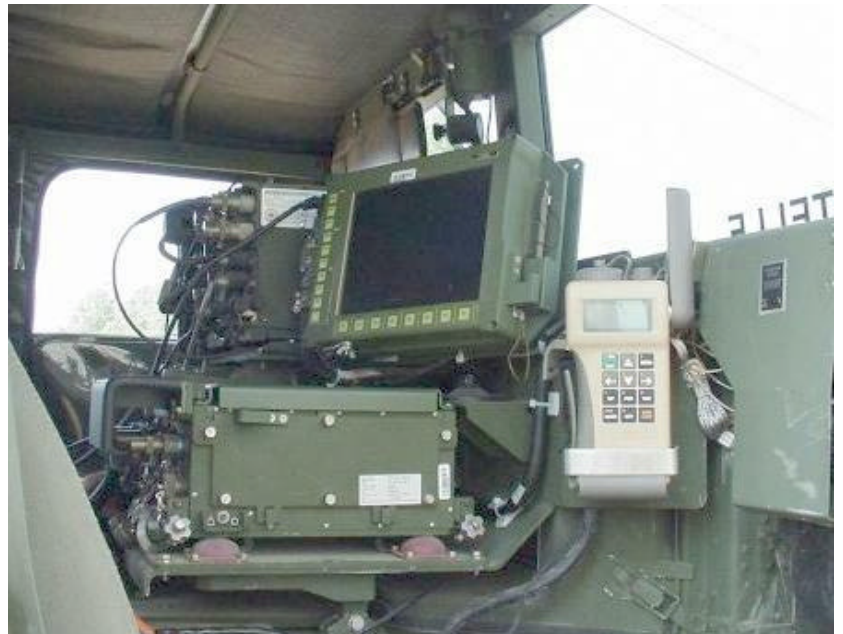
A FBCB2 Blue Force Tracking (BFT) vehicle installation with the PLGR receiver at right. PM GPS and PM FBCB2 are now working on a plan to replace the PLGR with embedded GPS (story below).
